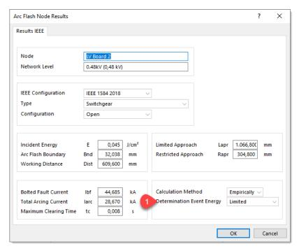
The field **Determination Event Energy** indicates whether adjustments have been made in determining the event energy (reduced arc current, current limitation of protection devices).
