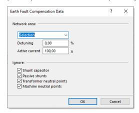
The **Detuning** v in the compensated network is the ratio of capacitive earth fault current  $I_c$  and the reactive current across the neutral point impedance  $I_{stp}$ .
