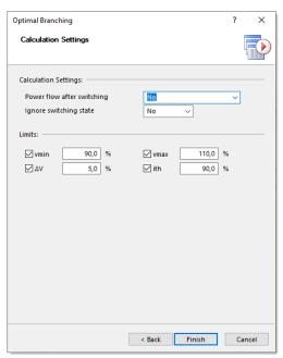
In the wizard it is also possible to define the control settings essential for the calculation module and
