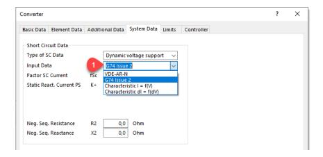
The **G74** Issue 2 option is new. The short-circuit current is determined interactively depending on the voltage at the connection node before and after the fault occurrence with the help of the rated current and the reactive current control characteristic. The rated current is determined with the rated apparent power and the rated voltage of the element.
