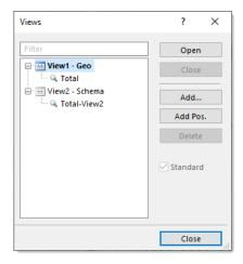
The network model may contain any number of additional views. One of them is the **standard view**. While the additional views can be opened and closed by the user as needed, this is not possible with the standard view. The standard view is always loaded when the network model is opened. Closing the standard view causes the network and all additional views to be closed. The standard view of the network model is set by activating the **Standard** option.
