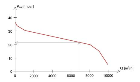
The input value is the flow Q across the pressure regulator determined by the steady-state iteration.
