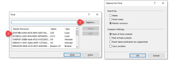
If the **Master resource** option is enabled, the display in the **Find** dialog box is changed (#2). Then only those elements of the network are displayed to which master resources are assigned. For each element the master resource, the name and the type are displayed.
