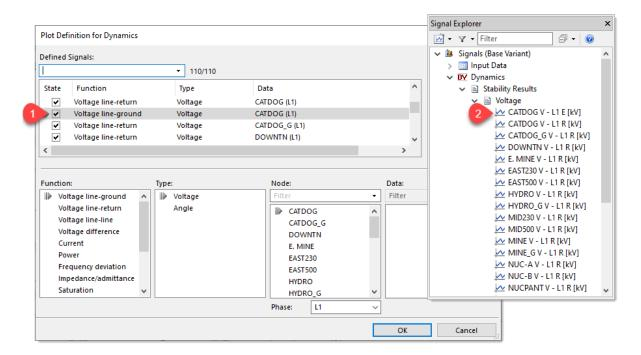
Now in the **Plot Definition for Dynamics** dialog box you can choose between the output of phase-to-ground voltages and phase-to-return voltages (#1). This differentiation in plotting is important for unbalanced network models as well as for those with isolated neutral points.
