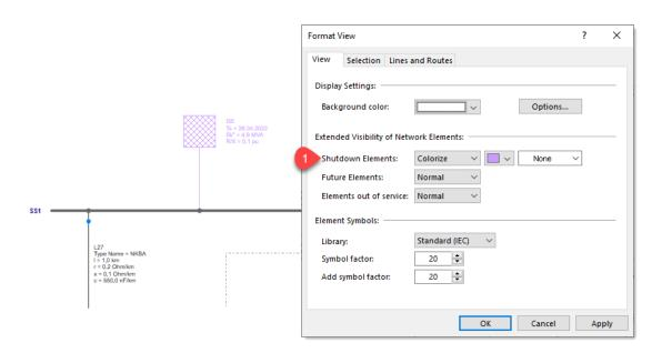
In this context, it is also new that as part of the textual representation of the input data of the network elements, the establishment and shutdown date can now also be shown in the view.
