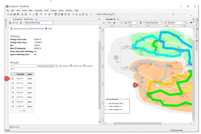
Another new functionality is the graphical visualization of the meshes in the network model. This visualization by highlighting (#2) can be activated in the **Options** dialog box in the **Results View**.
