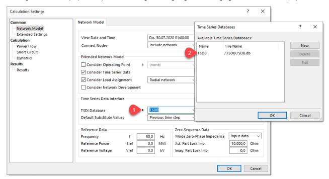
Also new is the option for extended predefinition of the **Default Substitute Values** when using the **Previous time step** option.
