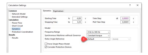
Due to the change, it is immediately visible in the Calculation Settings which settings are active for the rotor angle reference. In addition, it is easy to switch between the different options for different evaluations.
