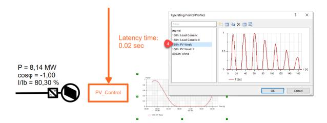
This new function also allows separate consideration of model levels for equipment, control and communication systems. In this way, the additional levels for control and communication signals can be superimposed or subimposed on the power level and set off against it in color. The connection to the input data and models behind it is given by the link.
