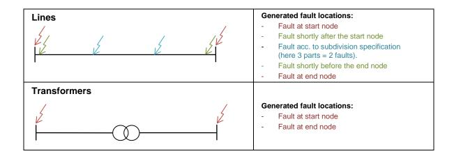
For each of these generated faults, the thermal stress of the network elements is checked. Here, the maximum possible thermal withstand of the network element must be greater than the determined thermal stress.
