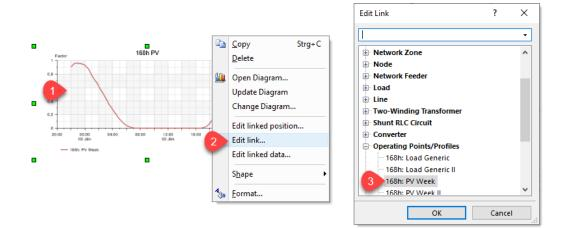
If network data is assigned, it will be displayed when you double-click the graphic object. In the example shown, profile data has been assigned. Therefore, the dialog box for editing operating points/profiles is opened here and the assigned data is selected.
