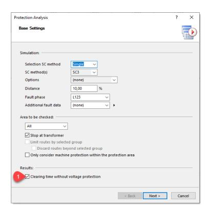
With the option **Clearing time without voltage protection**, the tripping of the voltage protection is not considered in the results in the clearing time. However, the pick-up and tripping during the fault clearing takes place with consideration of the voltage protection.
