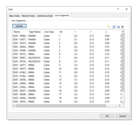
In the new tab, line segments can be added, removed and changed. Clicking the **Update** button updates the line data with the data determined from the line segments.
