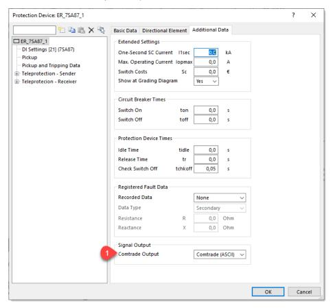
This generates an individual Comtrade file in the selected format (ASCII or binary) in the EMT simulation for all protection devices parameterized in this way. The secondary side signals of the assigned measurement transformers (currents and voltages) are automatically recorded in the file. The measurement transformer ratio is of course also stored in the Comtrade file. The generated Comtrade files are provided in the directory "xxx\_files\EXP":
