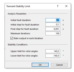
The results of the transient stability limit calculation are available in the message window in the HTML log. The log contains the individual states of each iteration with varied fault durations and at the end of the log the fault duration for the transition from "stable" to "unstable" is displayed.
