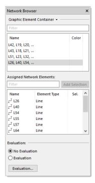
The new element container thus reduces the scope of information shown in the graphic view without losing flexibility in editing the network model or reducing the model. It is also possible to quickly switch the view style between the underlying complete network model representation (all information shown) to the style with the graphical element containers. For this purpose, the **Show Element Containers** option is available in the properties of the view.
