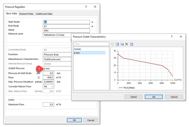
The output value for determining the outlet pressure is the flow Q at normal condition determined by the steady-state simulation.
