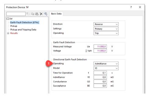
The new Admittance Method can be used with three different methods: Y0, G0 or B0.
