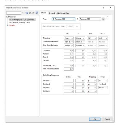
The implementation of the recloser in the protection simulation has also been extended. A switching sequence of the recloser that has been started (disconnection, pause time, reconnection) is now also run through if the fault is cleared by other protective devices during the switching sequence.
