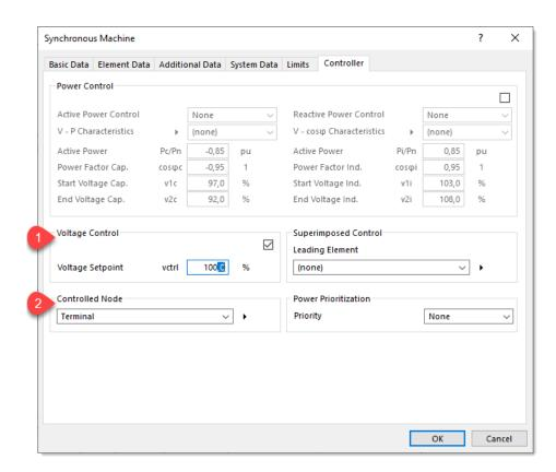
In the **Voltage Control (#1)** section, a target voltage can be specified for network feeders with the power flow type **active power and voltage**.
