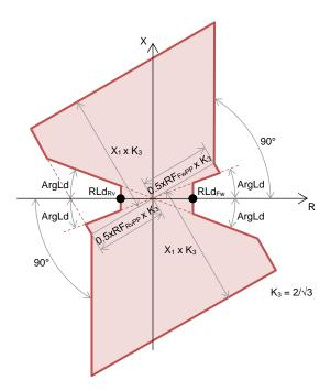
Pickup Area for Ground: The data for the resistance RN and reactance XN are determined via ground impedance factors. If no assignment is made, the specifications of distance zones are used.
