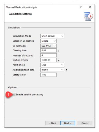
This automatically breaks down the calculation task into subtasks and distributes them to the computer's available calculation cores or those defined in the Options dialog box. The merging of the results also proceeds automatically.
