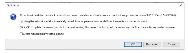
Here you have the possibility to update the client database by clicking **OK** or to disconnect it from the master database by clicking **Disconnect**. Then the client database is converted into a normal PSS SINCAL network.
