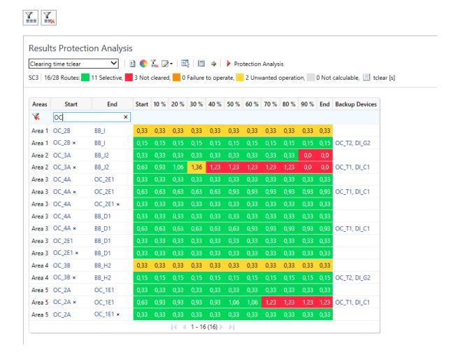
In the displayed input fields of the filter line, the criteria for reducing the displayed data can be entered. In the above picture, all protection routes are displayed where the name of the start or end device contains the character combination "OC".
