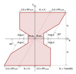
Pickup Area for the 3-Phase Fault: This special pickup area of the REL670 is used for 3-phase faults. Here the impedance pickup settings for phase in all directions are internally extended by a factor of  $2/\sqrt(3)$  and at the same time the surface is rotated 30° counterclockwise.
