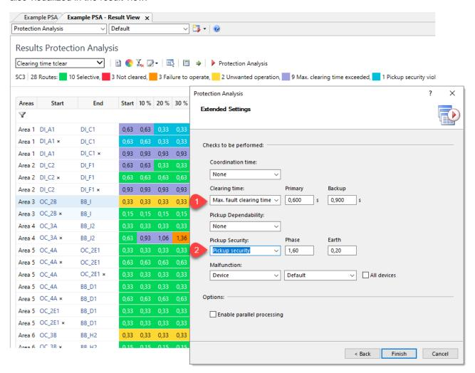
The check for **Pickup Security (#2)** has been extended. It is checked whether the maximum operating currents do not lead to a pickup when the specified factor is taken into account. The factor can now be specified separately for phase and ground and is taken into account accordingly in the calculation.
