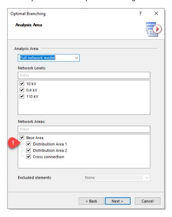
A new feature is that the **Network Areas** (#1) are offered for selection according to their hierarchical structure. This extension is available in all wizards where network areas are offered for selection.
