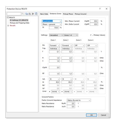
The pickup has been extensively revised. Now an individual impedance pickup is available for all distance protection devices modeled in PSS SINCAL. The selection of the adequate impedance pickup is done automatically when assigning the device type. The correct names of the settings are also displayed to match the device type.
