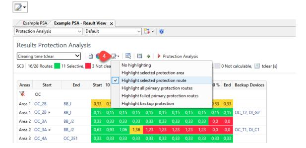
The row selected in the table (highlighted in blue) is thus automatically highlighted in the network graphic and when the row is changed, the highlighting is automatically adjusted.
