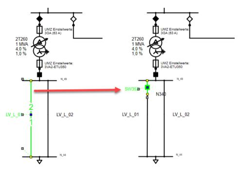
In the case that a large number of switches have to be inserted in existing network elements in a network model, the insert mode **Insert Switch** (e.g. can be activated in the **Toolbox**) is also available.
