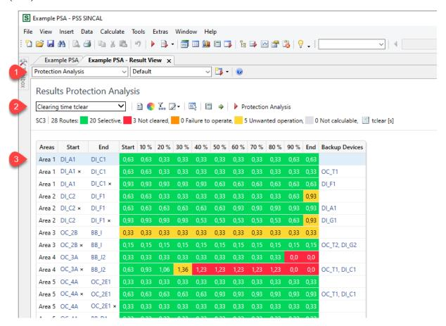
Primarily, the result view consists of a static window frame with a toolbar and the dynamic display area.
