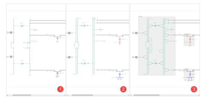
**Network model #1** shows a modeling concept without the use of switches. The implicitly available connection capability of a terminal in PSS SINCAL allows each network element to be switched using its terminal(s). For conceptual studies in the network model in early planning phases, this approach is sufficient and can be applied without the detailed planning of substations and outgoing sections.
