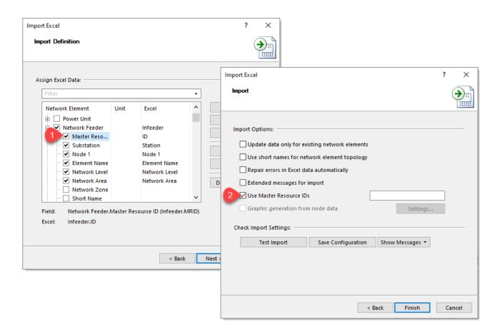
With the option **Use Master Resource IDs (#2)** the identification can be activated during import on master resource IDs instead of the topology assignment. The category of the master resource can be specified optionally via the associated input field. If no category is specified, all master resource IDs are used.
