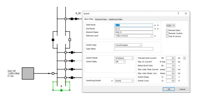
A switch element has the same topology data as all branch elements. The two **Terminals**, the **Element Name** and the **Network Level** can be defined. As with all network elements, there is also the **Element Data** tab, where further topological assignments to **Network Area**, **Network Zone** and **Substation** can be made and also the **Establishment Date** and **Shutdown Date** can be defined.
